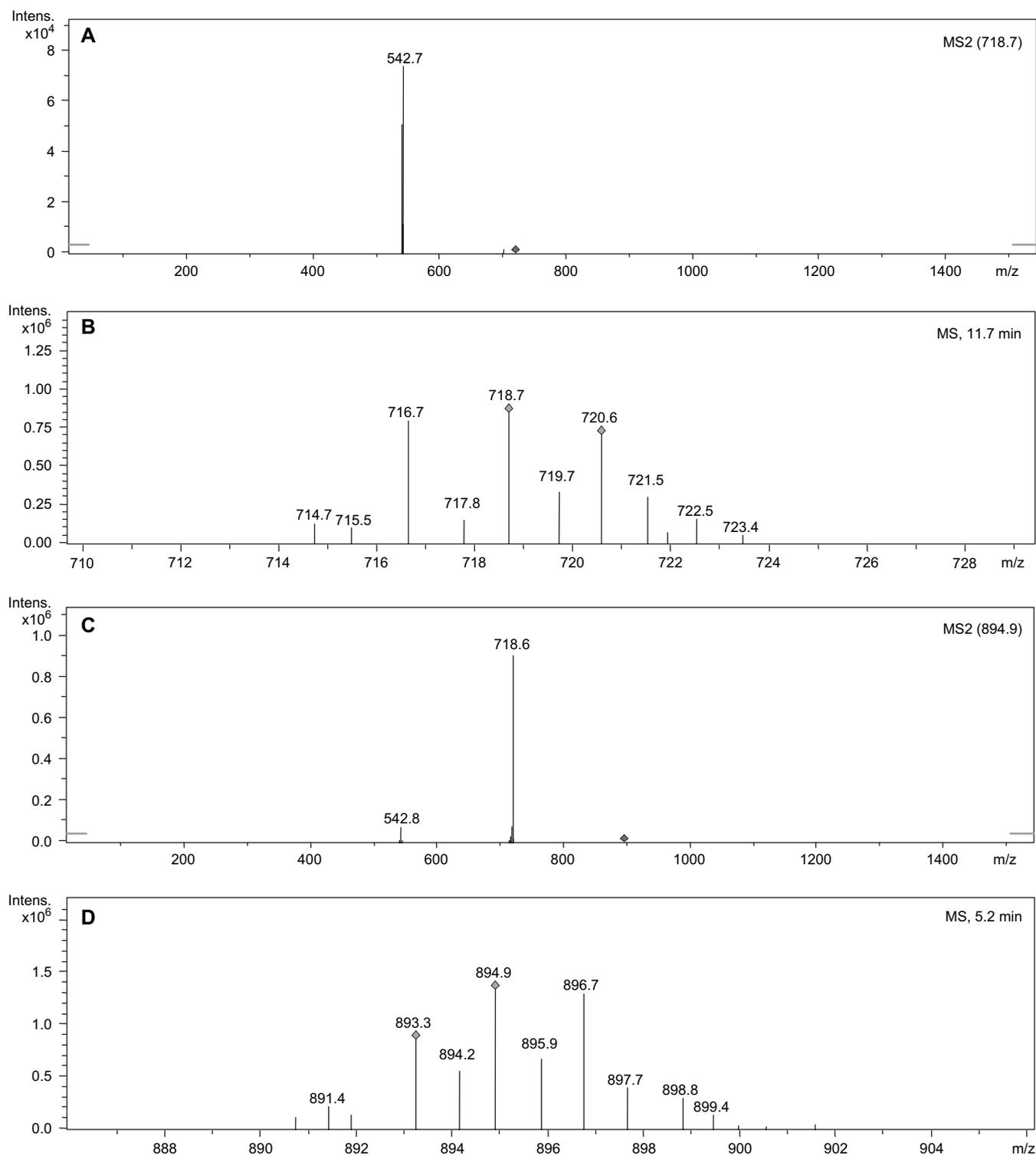
**FIG. 6.** Electrospray mass spectrum of TBBPA-glucuronide ([M-H] ion): (A) showing fragmentation of m/z 718 gives a loss of 176 amu; (B) isotope pattern of four bromine atoms. Electrospray mass spectrum of TBBPA-diglucuronide ([M-H] ion): (C) showing a fragmentation of m/z 895 gives a loss of  $2 \times 176$  amu, (D) isotope pattern of four bromine atoms.
